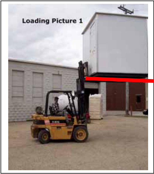
Fig. 1 - Picking Up By Tine Ports
