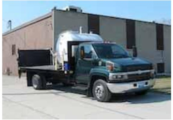
Pump Truck Lift Gate 600 Waste 250 internal Water Tank
