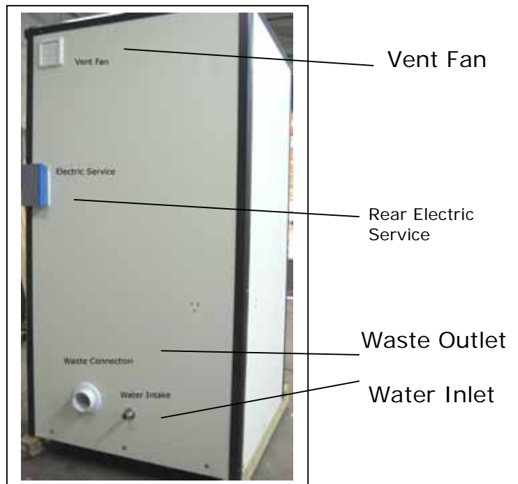
Fig. 8 Rear View Plumbing Connections
